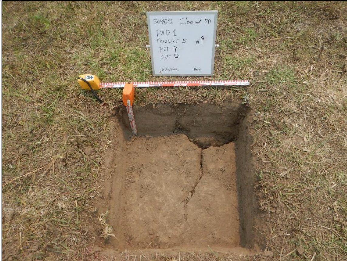
Plate 12 Soil profile in Transect 5 Pit 9, showing large clay shrink crack
